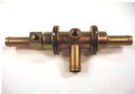
1H5-19 Overhauled, Vacuum Manifold Check Valve
