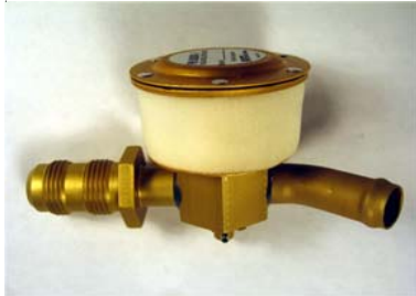
RA2H3-48 Vacuum Regulator AN-8 Threaded Fitting, Thread OD 7/8" (Pump), 5/8" Hose Fitting (instrument) Replaces - Airborne PN. 2H3-48, Aero Accessories PN. AA2H3-48
